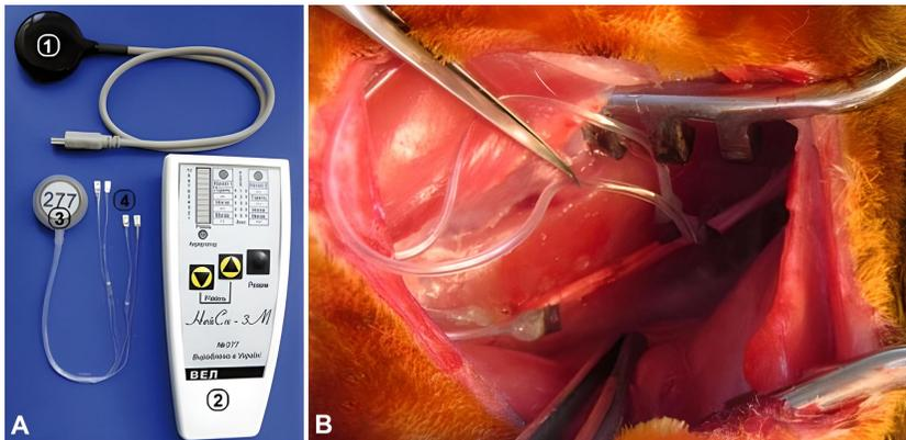
Fig. 1. NeySi-3M neurostimulator. A - general view. Nonimplantable part: 1. transmission antenna, 2. pulse generator unit (combined with the control panel); Implantable part: 3. receiving antenna, 4. electrodes. B - intraoperative photo: electrodes was fixed to the epineurium of sutured sciatic nerve.
