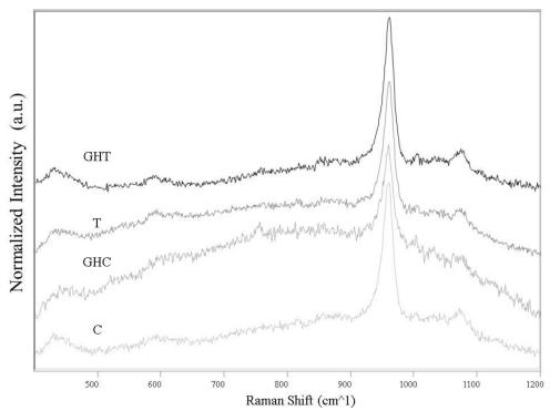
Fig. 2. Raman spectrum of bone 200 - 1200 cm-1. The intensity is demonstrated in arbitrary units (a.u.). The intensity of Y = 0 (offset correction function) normalized for better visualization of the bands. A 633nm laser was used.
