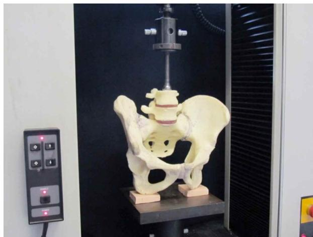
Fig. 1. Model of a pelvis coupled to an Instron 4502 Universal Testing Machine, with a 20 mm latex plate simulating the ischial tuberosities underlying tissue.
